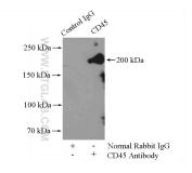
IP result of anti-CD45 (IP:20103-1-AP, 4ug; Detection:20103-1-AP 1:300) with mouse spleen tissue lysate 4800ug.
