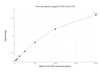
Standard curve of MP50057-1, CEACAM5 Monoclonal Matched Antibody Pair - BSA and Azide free measured by Sandwich ELISA. Capture antibody: 68675-1-PBS. Detection antibody: 68675-2-PBS (HRP conjugated). Standard: Eg0247. Range: 31.25-2000 pg/mL
