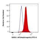
1X10^6 HeLa cells were intracellularly stained with 0.2 ug Anti-Human Amphiregulin (16036-1-AP) and CoraLite® 488-Conjugated Affini Pure Goat Anti-Rabbit IgG(IH+L) at dilution 1:1000 (red), or 0.2 ug Control Antibody. Cells were fixed with 4% PFA and permeabilized with Flow Cytometry Perm Buffer (PF00011-C). This data was developed using the same antibody clone with 16036-1-PBS in a different storage buffer formulation.
