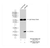
IP result of anti-ZNF580 (IP:25992-1-AP, 4ug; Detection:25992-1-AP 1:800) with COLO 320 cells lysate 1320 ug.
