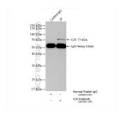
IP result of anti-ICK (IP:29728-1-AP, 4ug; Detection:29728-1-AP 1:400) with PC-3 cells lysate 1575 ug.
