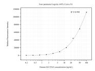
Cytometric bead array standard curve of MP50610-1, SLC25A3 Monoclonal Matched Antibody Pair, PBS Only. Capture antibody: 60451-1-PBS. Detection antibody: 60451-2-PBS. Standard:Ag4377. Range: 0.195-100 ng/mL
