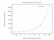
Cytometric bead array standard curve of MP50751-1, COX6B2 Monoclonal Matched Antibody Pair, PBS Only. Capture antibody: 60531-1-PBS. Detection antibody: 60531-2-PBS. Standard:Ag33133. Range: 0.391-100 ng/mL
