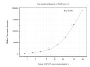
Cytometric bead array standard curve of MP50769-2, MRPL27 Monoclonal Matched Antibody Pair, PBS Only. Capture antibody: 60545-1-PBS. Detection antibody: 60545-3-PBS. Standard:Ag6870. Range: 0.781-100 ng/mL.
