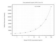
Cytometric bead array standard curve of MP51204-2, NUCB2 Monoclonal Matched Antibody Pair, PBS Only. Capture antibody: 60756-3-PBS. Detection antibody: 60756-4-PBS. Standard:Ag34234. Range: 0.781-100 ng/mL
