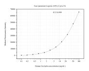
Cytometric bead array standard curve of MP51160-2, Occludin Monoclonal Matched Antibody Pair, PBS Only. Capture antibody: 66378-2-PBS. Detection antibody: 66378-3-PBS. Standard:Ag4057. Range: 0.098-100 ng/mL
