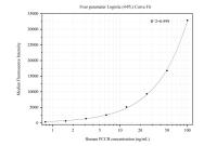
Cytometric bead array standard curve of MP50335-1, PCCB Monoclonal Matched Antibody Pair, PBS Only. Capture antibody: 66501-2-PBS. Detection antibody: 66501-3-PBS. Standard:Ag1608. Range: 1.563-100 ng/mL
