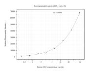
Cytometric bead array standard curve of MP51164-1, CD21 Monoclonal Matched Antibody Pair, PBS Only. Capture antibody: 66701-2-PBS. Detection antibody: 66701-3-PBS. Standard:Ag18058. Range: 0.391-50 ng/mL
