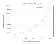
Cytometric bead array standard curve of MP50929-2, CFTR Monoclonal Matched Antibody Pair, PBS Only. Capture antibody: 66928-4-PBS. Detection antibody: 66928-3-PBS. Standard:Ag27810. Range: 3.125-100 ng/mL
