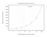
Cytometric bead array standard curve of MP51032-3, Myogenin Monoclonal Matched Antibody Pair, PBS Only. Capture antibody: 67082-1-PBS. Detection antibody: 67082-4-PBS. Standard:Ag6414. Range: 1.563-100 ng/mL
