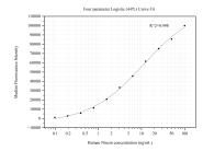
Cytometric bead array standard curve of MP50497-1, Ninein Monoclonal Matched Antibody Pair, PBS Only. Capture antibody: 67132-2-PBS. Detection antibody: 67132-3-PBS. Standard:Ag14652. Range: 0.098-100 ng/mL
