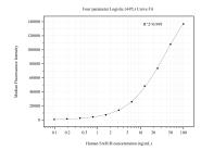
Cytometric bead array standard curve of MP50803-1, SAR1B Monoclonal Matched Antibody Pair, PBS Only. Capture antibody: 67765-2-PBS. Detection antibody: 67765-3-PBS. Standard:Ag7718. Range: 0.098-100 ng/mL
