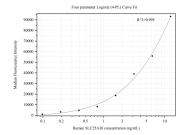
Cytometric bead array standard curve of MP50339-1, SLC25A36 Monoclonal Matched Antibody Pair, PBS Only. Capture antibody: 67896-2-PBS. Detection antibody: 67896-3-PBS. Standard:Ag23894. Range: 0.098-12.5 ng/mL
