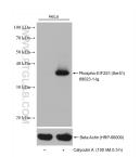
Non-treated and Calyculin A treated HeLa cells were subjected to SDS PAGE followed by western blot with 68023-1-1g (Phospho-EIF2S1 (Ser51) antibody) at dilution of 1:20000 incubated at room temperature for 1.5 hours. The membrane was stripped and re-blotted with Beta Actin (HRP-66009) antibody as loading control. This data was developed using the same antibody clone with 68023-1-PBS in a different storage buffer formulation.
