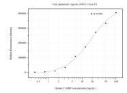
Cytometric bead array standard curve of MP50719-1, C1QBP Monoclonal Matched Antibody Pair, PBS Only. Capture antibody: 68084-2-PBS. Detection antibody: 68084-3-PBS. Standard:Ag19773. Range: 0.391-100 ng/mL
