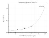
Sandwich ELISA standard curve of MP50025-1, RTN3 Monoclonal Matched Antibody Pair, PBS Only. Capture antibody: 68215-2-PBS. Detection antibody: HRP-conjugated 68215-1-PBS. Standard: Ag13766. Range: 0.625-20 ng/mL
