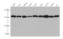
Various lysates were subjected to SDS PAGE followed by western blot with 68316-1-lg (Ataxin 2 antibody) at dilution of 1:5000 incubated at room temperature for 1.5 hours. This data was developed using the same antibody clone with 68316-1-PBS in a different storage buffer formulation.
