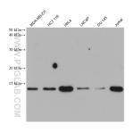
Various lysates were subjected to SDS PAGE followed by western blot with 68408-1-lg (ISG15 antibody) at dilution of 1:5000 incubated at room temperature for 1.5 hours. This data was developed using the same antibody clone with 68408-1-PBS in a different storage buffer formulation.
