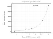
Cytometric bead array standard curve of MP51098-2, IGF2BP3 Monoclonal Matched Antibody Pair, PBS Only. Capture antibody: 68470-4-PBS. Detection antibody: 68470-3-PBS. Standard:Ag6349. Range: 0.781-50 ng/mL
