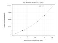
Cytometric bead array standard curve of MP50870-2, TEX264 Monoclonal Matched Antibody Pair, PBS Only. Capture antibody: 68507-2-PBS. Detection antibody: 68507-3-PBS. Standard:Ag33710. Range: 0.098-100 ng/mL
