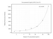
Cytometric bead array standard curve of MP50548-5, LTF Monoclonal Matched Antibody Pair, PBS Only. Capture antibody: 68509-2-PBS. Detection antibody: 68509-4-PBS. Standard:Ag33645. Range: 1.563-100 ng/mL
