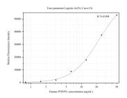
Cytometric bead array standard curve of MP50287-1, PTPIP51 Monoclonal Matched Antibody Pair, PBS Only. Capture antibody: 68582-2-PBS. Detection antibody: 68582-3-PBS. Standard:Ag15135. Range: 0.781-50 ng/mL
