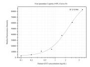
Cytometric bead array standard curve of MP50251-2, GS15 Monoclonal Matched Antibody Pair, PBS Only. Capture antibody: 68856-1-PBS. Detection antibody: 68856-3-PBS. Standard:Ag5506. Range: 0.098-6.25 ng/mL
