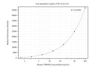
Cytometric bead array standard curve of MP50261-2, TIMM8A Monoclonal Matched Antibody Pair, PBS Only. Capture antibody: 68866-1-PBS. Detection antibody: 68866-3-PBS. Standard:Ag33190. Range: 1.563-100 ng/mL.
