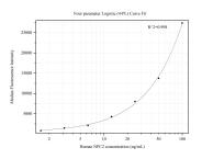
Cytometric bead array standard curve of MP50350-1, NPC2 Monoclonal Matched Antibody Pair, PBS Only. Capture antibody: 68927-1-PBS. Detection antibody: 68927-2-PBS. Standard:Ag34710. Range: 1.563-100 ng/mL
