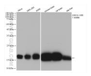
Various lysates were subjected to SDS PAGE followed by western blot with 81615-1-RR (pan-RAS antibody) at dilution of 1:50000 incubated at room temperature for 1.5 hours. This data was developed using the same antibody clone with 81615-1-PBS in a different storage buffer formulation.
