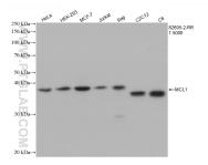
Various lysates were subjected to SDS PAGE followed by western blot with 82695-2-RR (MCL1 antibody) at dilution of 1:5000 incubated at room temperature for 1.5 hours. This data was developed using the same antibody clone with 82695-2-PBS in a different storage buffer formulation.
