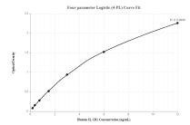
Sandwich ELISA standard curve of MP00062-1, IL-1R1 Recombinant Matched Antibody Pair, PBS Only. Capture antibody: 82990-2-PBS. Detection antibody: 82990-1-PBS. Standard: Ag25998. Range: 0.188-12 ng/mL
