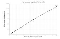
Cytometric bead array standard curve of MP00135-3, KIAA0776 Recombinant Matched Antibody Pair, PBS Only. Capture antibody: 83047-1-PBS. Detection antibody: 83047-2-PBS. Standard: Ag23362. Range: 0.625-20 ng/mL
