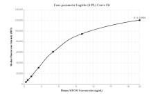
Cytometric bead array standard curve of MP00254-1, MTCO2 Recombinant Matched Antibody Pair, PBS Only. Capture antibody: 83132-3-PBS. Detection antibody: 83132-6-PBS. Standard: SY01099. Range: 0.313-20 ng/mL
