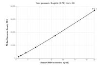
Cytometric bead array standard curve of MP00200-2, GBX2 Recombinant Matched Antibody Pair, PBS Only. Capture antibody: 83145-3-PBS. Detection antibody: 83145-4-PBS. Standard: Ag16288. Range: 0.625-20 ng/mL
