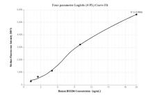
Cytometric bead array standard curve of MP00150-1, HOXB6 Recombinant Matched Antibody Pair, PBS Only. Capture antibody: 83155-1-PBS. Detection antibody: 83155-2-PBS. Standard: Ag14189. Range: 1.25-20 ng/mL
