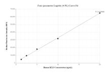
Cytometric bead array standard curve of MP00207-1, RELN Recombinant Matched Antibody Pair, PBS Only. Capture antibody: 83233-1-PBS. Detection antibody: 83233-2-PBS. Standard: SY00905. Range: 1.25-20 ng/mL
