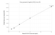
Cytometric bead array standard curve of MP00164-3, KCN 115 Recombinant Matched Antibody Pair, PBS Only. Capture antibody: 83257-1-PBS. Detection antibody: 83257-3-PBS. Standard: Ag34655. Range: 2.5-40 ng/mL
