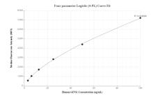
Cytometric bead array standard curve of MP00317-2, GINS1 Recombinant Matched Antibody Pair, PBS Only. Capture antibody: 83293-2-PBS. Detection antibody: 83293-1-PBS. Standard: Ag8895. Range: 3.13-100 ng/mL
