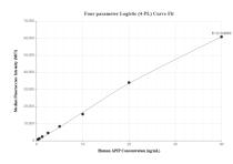
Cytometric bead array standard curve of MP00346-2, APIP Recombinant Matched Antibody Pair - BSA and Azide Free. Capture antibody: 83320-4-PBS. Detection antibody: 83320-1-PBS. Standard: Ag2729. Range: 0.313-40 ng/mL
