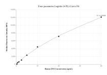
Cytometric bead array standard curve of MP00751-3, EPO Recombinant Matched Antibody Pair, PBS Only. Capture antibody: 83762-1-PBS. Detection antibody: 83762-4-PBS. Standard: Eg0197. Range: 0.313-40 ng/mL
