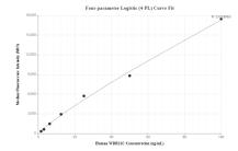
Cytometric bead array standard curve of MP00738-2, WDR21C Recombinant Matched Antibody Pair, PBS Only. Capture antibody: 83802-1-PBS. Detection antibody: 83802-4-PBS. Standard: Ag30748. Range: 1.56-100 ng/mL
