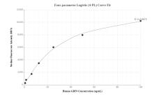
Cytometric bead array standard curve of MP00911-1, GDF9 Recombinant Matched Antibody Pair, PBS Only. Capture antibody: 83956-2-PBS. Detection antibody: 83956-1-PBS. Standard: Ag29603. Range: 0.781-100 ng/mL
