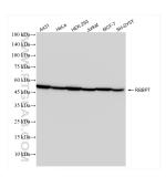
Various lysates were subjected to SDS PAGE followed by western blot with 84330-1-RR (RBBP7 antibody) at dilution of 1:10000 incubated at room temperature for 1.5 hours. This data was developed using the same antibody clone with 84330-1-PBS in a different storage buffer formulation.
