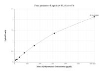
Sandwich ELISA standard curve of MP01284-4, Mouse MPO Recombinant Matched Antibody Pair -PBS only. 84436-3-PBS was coated to a plate as the capture antibody and incubated with serial dilutions of standard Eg0702. 84436-4-PBS was HRP conjugated as the detection antibody. Range: 9.77-625 pg/mL
