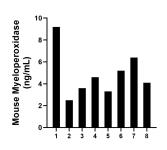
Serum of eight mice was measured. The mouse Myeloperoxidase concentration of detected samples was determined to be 4.86 ng/mL with a range of 2.54 - 9.19 ng/mL
