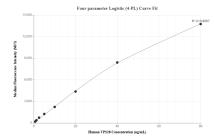
Cytometric bead array standard curve of MP01354-1, VP528 Recombinant Matched Antibody Pair, PBS Only. Capture antibody: 84472-1-PBS. Detection antibody: 84472-2-PBS. Standard: Ag7784. Range: 0.625-80 ng/mL
