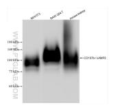
Various lysates were subjected to SDS PAGE followed by western blot with 84474-5-RR (CD107b / LAMP2 antibody) at dilution of 1:10000 incubated at room temperature for 1.5 hours.
