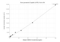
Cytometric bead array standard curve of MP01457-2, CORO 1A Recombinant Matched Antibody Pair, PBS Only. Capture antibody: 84602-2-PBS. Detection antibody: 84602-3-PBS. Standard: Ag12139. Range: 0.781-100 ng/mL.
