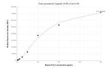
Cytometric bead array standard curve of MP01520-1, WASP Recombinant Matched Antibody Pair, PBS Only. Capture antibody: 84714-1-PBS. Detection antibody: 84714-2-PBS. Standard: Ag1444. Range: 0.625-80 ng/mL
