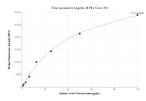
Cytometric bead array standard curve of MP01551-2, ACS52 Recombinant Matched Antibody Pair, PBS Only. Capture antibody: 84774-4-PBS. Detection antibody: 84774-2-PBS. Standard: Ag9121. Range: 0.781-100 ng/mL
